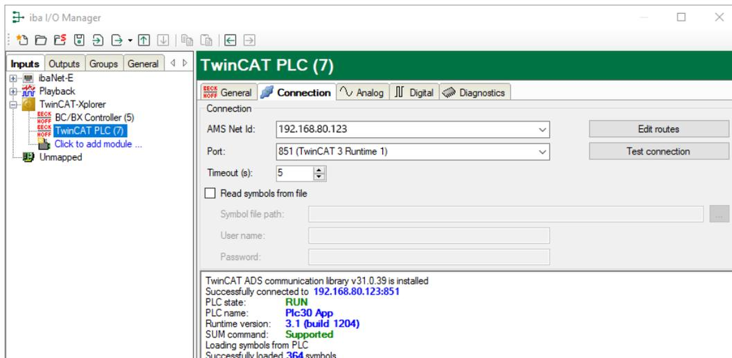
If the symbols are not stored on the PLC, which is the case for bus controllers, then a symbol file needs to be specified. The symbol file is a TPY file that is generated by the TwinCAT compiler. It is normally located in the same directory as the project file. The *ibaPDA* service is going to access the symbol file. This means that if the symbol file is located on a network share then you need to specify the UNC path and proper user credentials for it.
