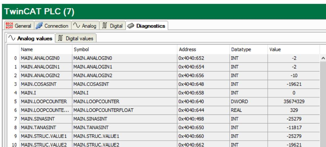
The screenshot shows the 'Diagnostics' tab of the TwinCAT PLC (7) interface. It displays a table of signal values. The table has columns for Name, Symbol, Address, Datatype, and Value. The table is divided into 'Analog values' and 'Digital values' sections. The 'Analog values' section is active, showing a list of signals with their current values. Some rows are highlighted in grey, indicating they are inactive.
