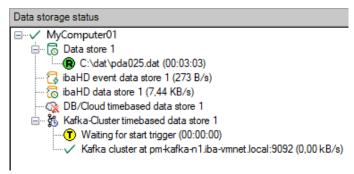
All defined data stores and their respective status are displayed here, depending on the data store, with server address, acquisition duration, write speed, etc.
