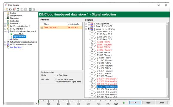
In the profile list, select the storage profile to which you want to assign certain signals. Set a check mark in the selection fields next to the signals which you would like to assign to this profile. A signal can only be assigned to one profile per data store.
