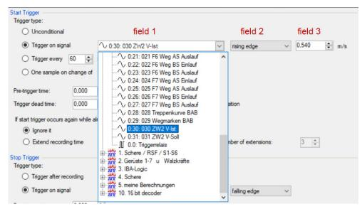
Depending on whether a digital or an analog signal was selected, the fields 2 or 3, respectively, are offered allowing the trigger event to be defined more specifically.
