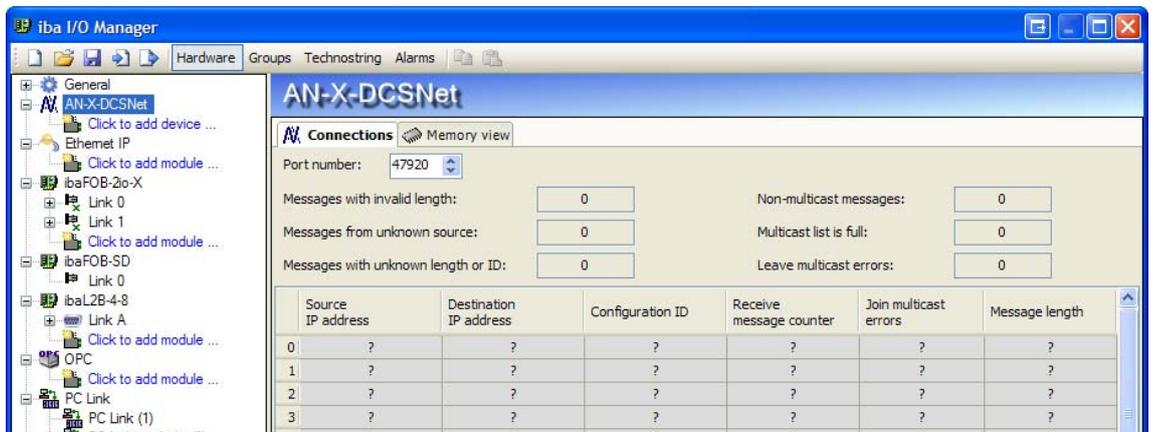
On the interface you can setup the UDP port number that ibaPDA listens to for messages from an AN-X-DCSNet device. Normally the default port number of 47920 is ok. The connections grid shows the current connections to AN-X-DCSNet devices. There are also some error counters on the interface. Check out chapter 3 for more information about these counters and the connections grid.
